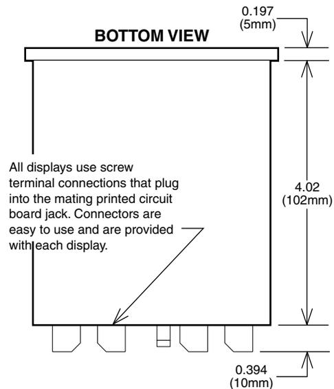
All displays use screw terminal connections that plug into the mating printed circuit board jack. Connectors are easy to use and are provided with each display.
